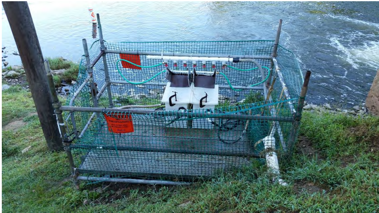
Figure 3.1-4: Manifold for Garden Hose Supply Lines for Attraction Flows, Octoraro Creek, 2016
